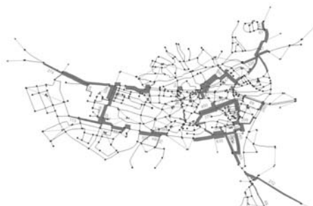
Photo 2: Counted values for cars on intersections, calculate in Visum, presented in sections
